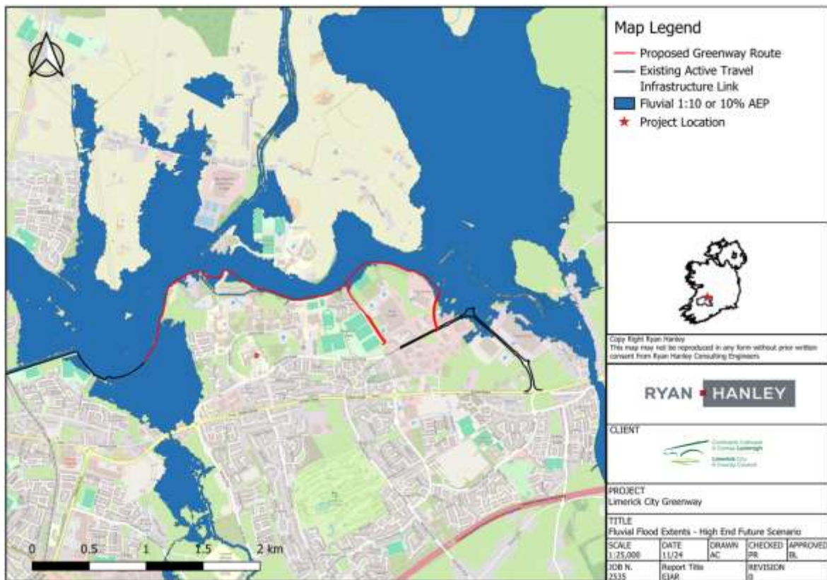
Figure 8-13 High End Future flood risk, high probability (i.e. 10% AEP) event flood extents
