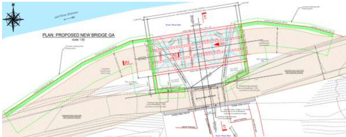
Figure 4-90: Plan for the proposed new bridge 2 alongside the existing stone bridge (refer to drawing RHA-XX-DR-S-SP0021)
